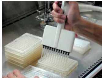
Add the plasmid/reagent solution into each well. (25 \mu L/well)
